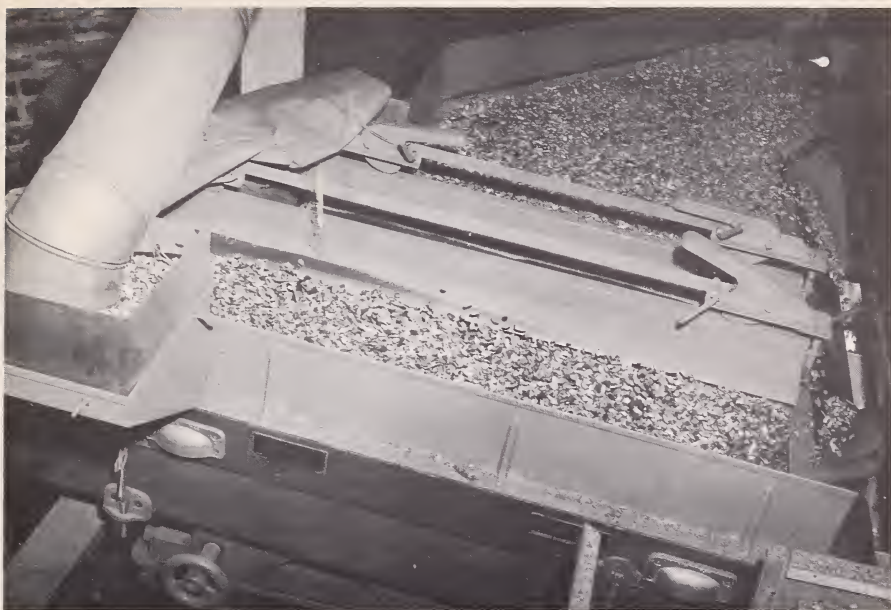
FIGURE 15.—An oscillating shaker screen separator removes foreign material from kernels. This machine is usually set up so that the stock can be run over it more than once if necessary.
